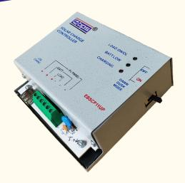
**DUSK TO DAWN**: Switch is kept ON then dusk to dawn mode is selected. With this mode turned ON Load is connected when sunlight is not present and load is turned OFF when solar is present. **Normal Mode**: Switch is kept OFF than Normal mode is selected.
